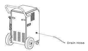
• If the drain area is located above the Dehumidifier, the maximum capacity of the water pump is 16.4 ft (5 m). If the water is drained downwards, there is no limit for the distance.
